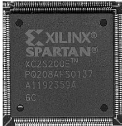
**Figure L1.2:** The Xilinx Spartan-2E FPGAs have the model number (XC2S200E), package type (PQ208), and speed grade (6) printed on the top of the chip.
